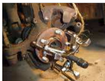
3 Jaw Puller used for removing tyre hub
