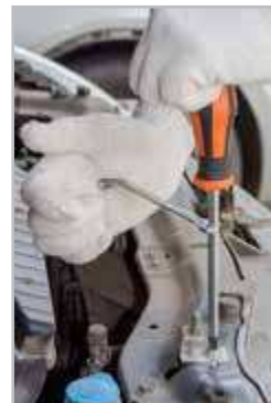
Hex shaft can be tightened using a spanner for high torque applications
