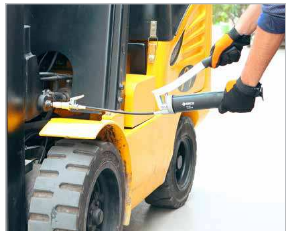
HANDS FREE OPERATION Coupler need not be held during greasing
