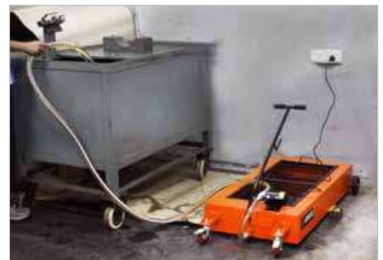
Extracting oil from the truck drain using AC power motor
