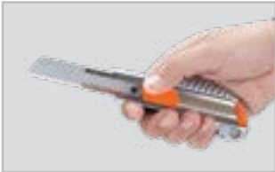
Slide the lever to retract the blade
