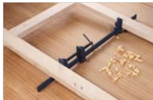
Duo Bar used for internal clamping
