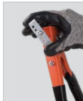
Convenient change of nose pieces with wrench
