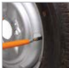
Prying wheel balancing weights from the alloy rims
