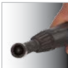
Welding Gun Nozzle filled with weld splatter
