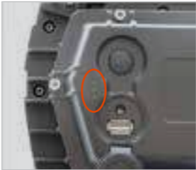
3 LED battery level indicator
