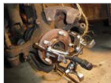
3 Jaw Puller used for removing tyre hub
