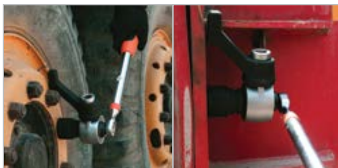
Foot reaction bar for obstacles at short distance
