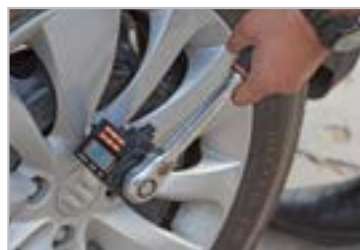
MODE 1 Use as digital torque adaptor
